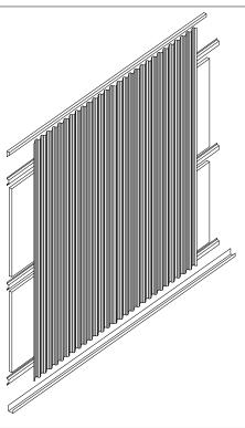
**Description:** Corrugated metal wall panel. Panels are attached to concealed hat channel,
